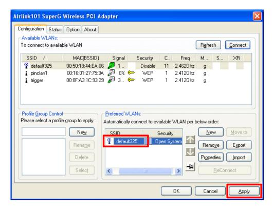
**Note:** Be sure to remove the wrong SSID from the **Preferred WLANs** box before adding any new SSID. You can remove the wrong SSID by selecting it and clicking on **Remove**.
